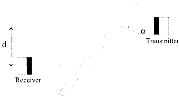
Figure 12 Experimental configuration for the detection of a Lamb mode
