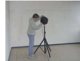
Omnidirectional source and reverberant room
