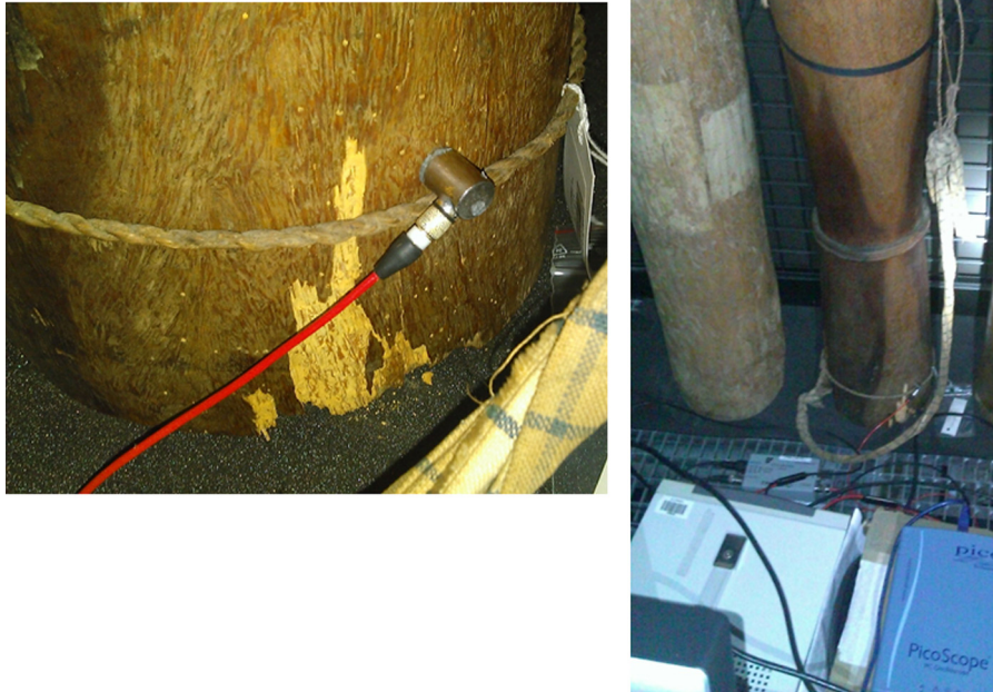
Fig. 5. African drum equipped with the acoustic emission (AE) set up.
