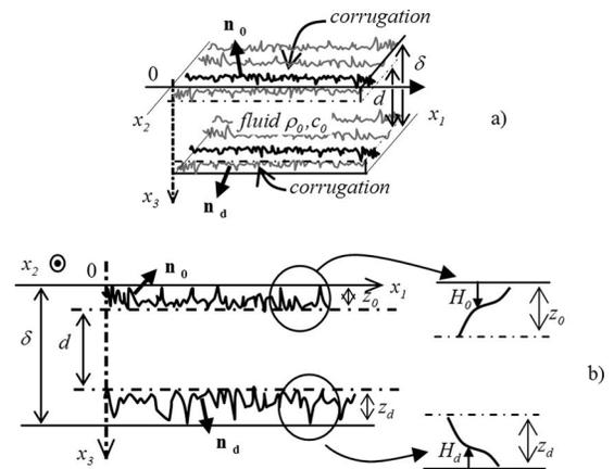
FIG. 1. Fluid plate between two perturbed boundary surfaces.
