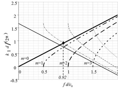
FIG. 2. Dispersion curves (thick lines) of the guide with smooth interfaces ( $k_{x_1} d/(2\pi) = \sqrt{(fd/c_0)^2 - (m/2)^2}$ ) and curves (thin lines) corresponding to the phonon relation (11) ( $k_{x_1} d/(2\pi) = d/\Lambda - \sqrt{(fd/c_0)^2 - (m/2)^2}$ ). Solid lines: mode  $m=0$ , dash-dots lines: mode  $m=1$ , dashed lines:  $m=2$ , dotted lines:  $m=3$ .
