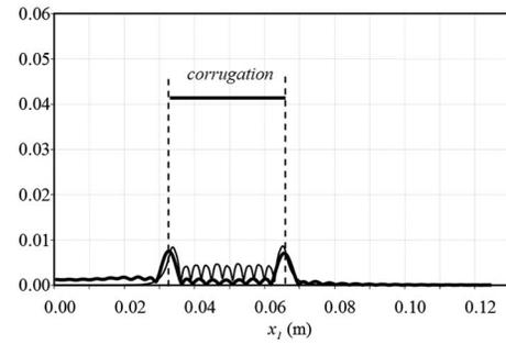
FIG. 8. Modulus of the normalized amplitude of the evanescent modes of the pressure variation for the sawtooth profile shown in Fig. 6 when  $fd/c_0=0.91$  (i.e.,  $f=1.06$  MHz). Thick solid line: result obtained from ATILA finite element code, thin solid line: result obtained from the analytical intermodal shape profile model at the third order for the evanescent mode  $\mu=2$ .
