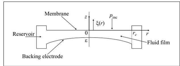
Figure 1. Schematic view of a miniaturized microphone with a non planar backing electrode and a peripheral reservoir.
