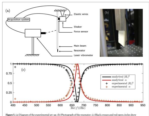
respectively  $|R_r|^2$  and  $\alpha_r$  for the critical coupled configuration measured with the experimental set-up. Black dashed and red continuous lines show  $|R_r|^2$  and  $\alpha_r$  calculated with the analytical model.
