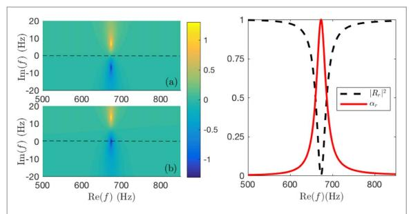
**Figure 3.** Representation of the perfect absorption for the reflection problem. (a), (b) Show the representation of the  $\log_{10}(|R_r|)$  for the lossless and lossy configurations respectively. (c) Red continuous and black dashed lines show the analytical absorption and reflection coefficients for the critical coupled configuration respectively.
