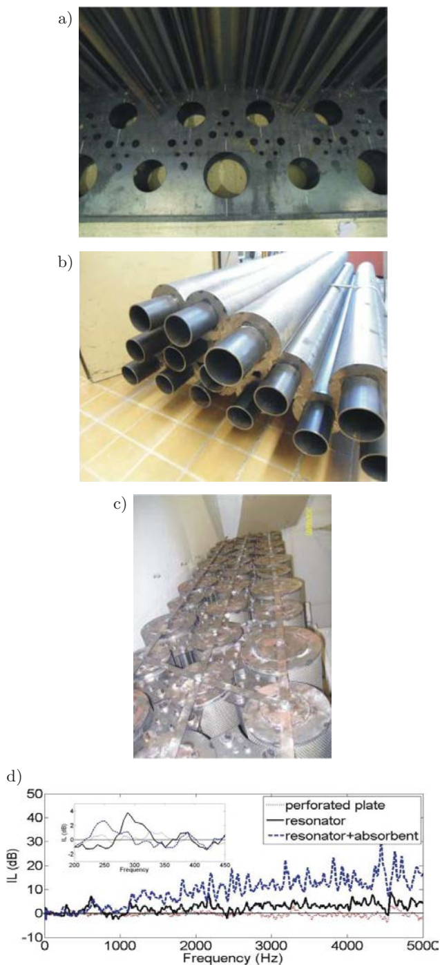
Fig. 3. Different details of the FSCAB used in the standardization process; a) placement of the scatterers in the fastening system; b) detail of the hard core of the cylinders used; c) constructive detail of the system showing the assembly among the top of the scatterers; d) IL spectra of the different materials and combinations that form the multi-phenomena scatterers obtained in anechoic chamber.
