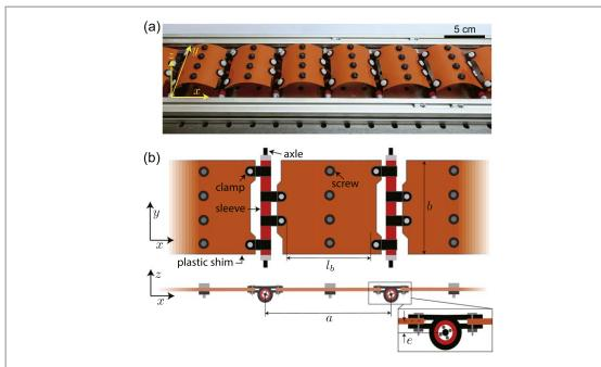
Figure 1. (a) Our system consists of a chain of pin-joined precompressed elastic beams. (b) Schematic of our system. Both top view and side view are shown.
