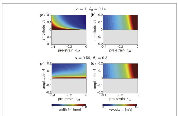
**Figure 5.** Analytically predicted evolution of the width W and the velocity c as a function of the amplitude A and the applied pre-strain  $\varepsilon_{\rm st}$  for a chain characterized by (a), (b)  $\alpha=1$  and  $\theta_0=0.14$  and (c), (d)  $\alpha=0.56$  and  $\theta_0=0.3$ . The gray area highlights the region in which the width predicted by the continuum model is imaginary, so that the solitary wave solution is not valid.
