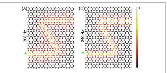
**Figure 6.** Steady state of pressure field in a finite size network having a *Z*-shape interface by connecting two SLGNs with free zigzag edges. The position of input source is marked by a yellow arrow. (a) Input sound wave frequency is 208 Hz. (b) Input sound wave frequency is 240 Hz.
