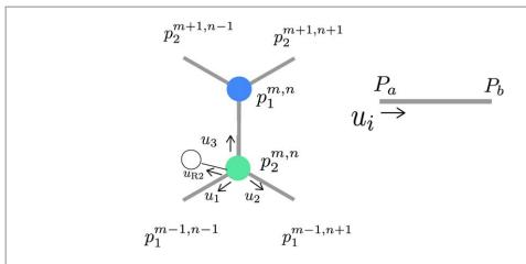
Figure A1. Schematic presentation of an unit cell of the graphene network loaded with a single Helmholtz resonator. Sketch of monomodes propagation in a waveguide is presented in the right.
