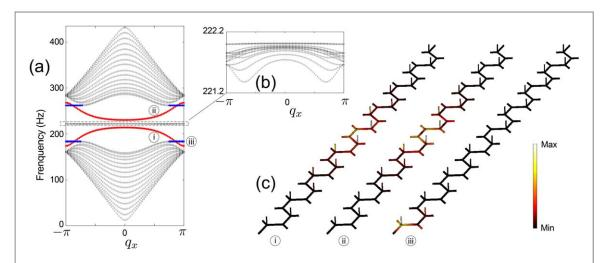
Figure 5. (a) Dispersion of SLGN with an interface composed of two free zigzag edges. The red (blue) dots highlight the interface (edge) mode branches. (b) Close view of the nearly flat region in (a). (c) Pressure field distributions of eigenmodes of the three bands in (a).
