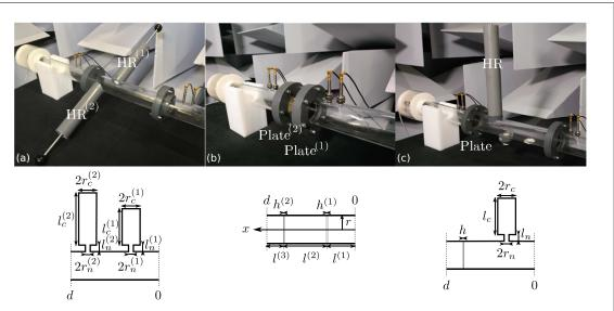
**Figure 1.** Pictures of the three studied Willis unit cells: (a) a straight duct loaded by two detuned HR located at different positions, (b) a straight duct with two detuned plates clampled in it, and (c) a straight duct loaded by an HR and with a plate clamped in it at a different position. A sketch of the configuration is provided below each picture.
